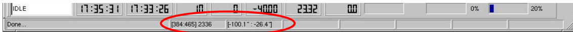
Figure 13. Information obtained by clicking the left mouse button over the image: location, number of counts and position in arc seconds
