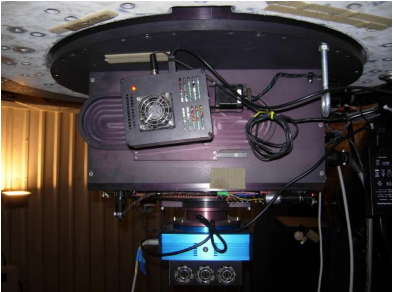
FIGURE 6-2 DUAL FILTER WHEEL & X-STAGE GUIDER INSTRUMENT
