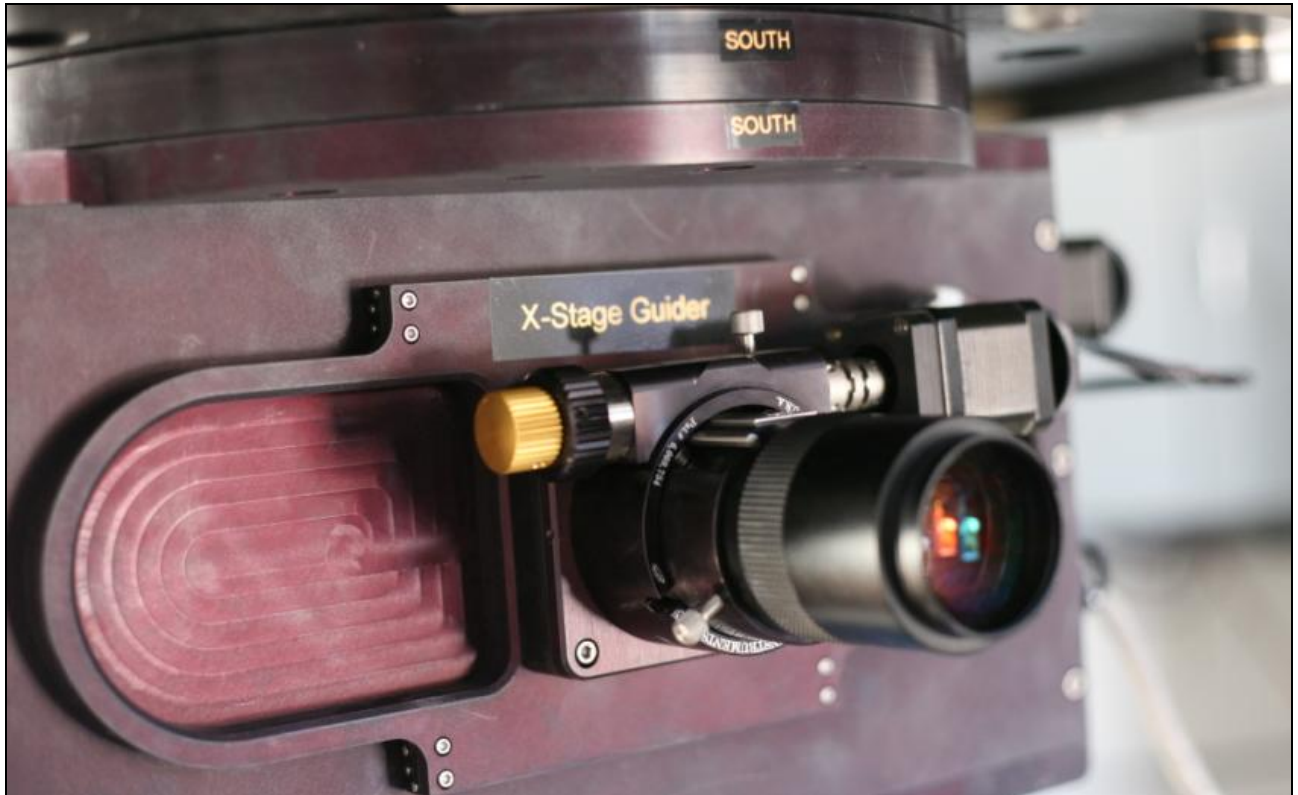
FIGURE 6-3 X-STAGE CENTERED WITH EYEPIECE INSTALLED
